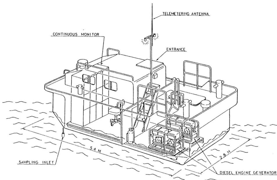
Fig. 1. Continuous water quality monitoring system
